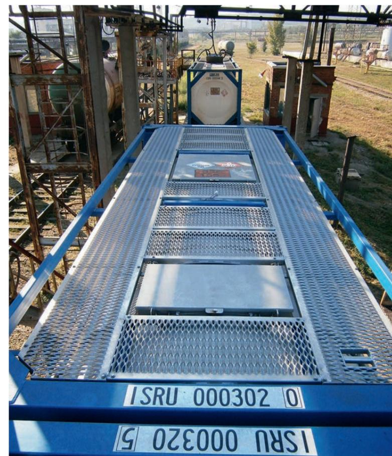
with shut-off valves and valves are closed with a cover. The top surface of the tank container is fully equipped with metal tracks, which keeps the container itself from damage and provides convenient loading and moving around the container. Tank containers are equipped with pressure gauges (pressure sensors) and pressure relief valves.
